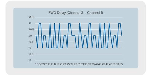
The results indicate a 20ns delay difference consistent with the 4m of added fiber.
