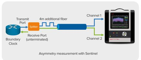
Sentinel measures the forward delay  $(T_2-T_1)$  on channel 1 and 2. The two delays are displayed, and the difference can be observed. The measurement data has also been downloaded and graphed below.
