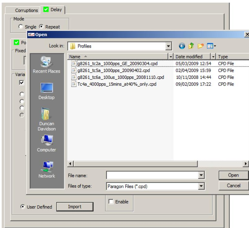
10. For adding the same or different delays in the other direction. Select the other direction tab and follow steps 4 to 9 above. When delays are being added in both directions –there will be a green tick shown in each direction tab as shown below.
