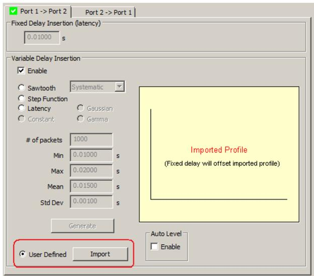
9. Navigate to the folder where the desired profile is, select it and click Open. The profile will be imported and a status bar will show the progress of the import.
