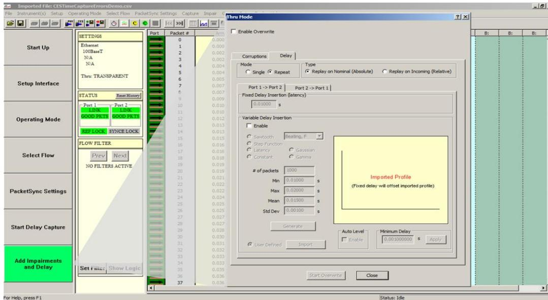
It is possible to add lost/errored packets at the same time a delay is being applied to the packets.
