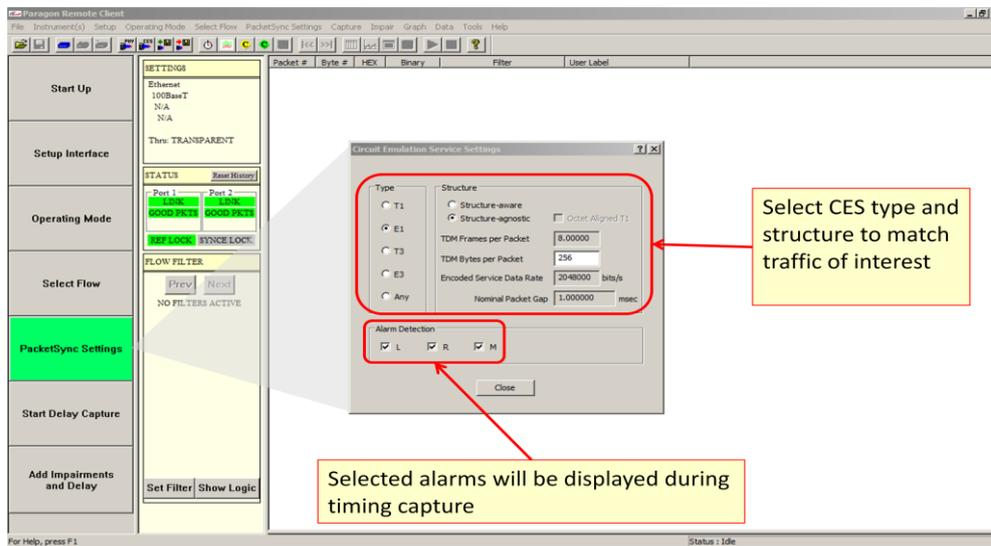
2. Select the appropriate Type and Structure to match your flow of interest. Note: it is essential that the resulting Nominal Packet Gap is the same as your traffic flow, for accurate TIE calculations.
