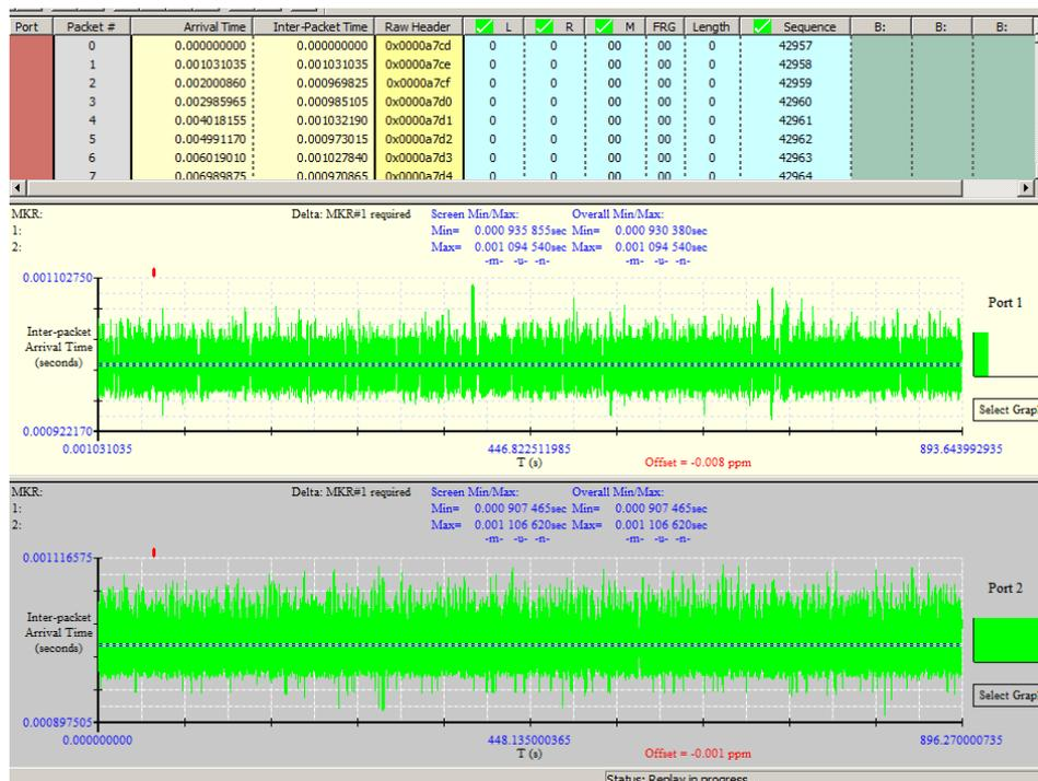
The replayed profile for each direction is displayed. The Header and timing will show the data for the active graph which is shown in white. To change between graphs, click the graph that is required.
