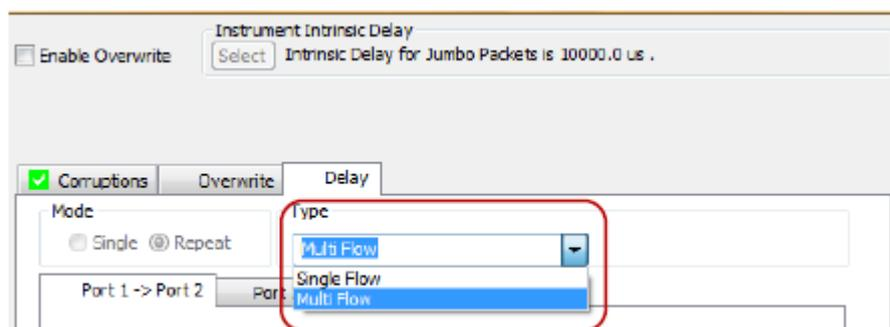
The selection of Single Flow maintains the existing method of applying the delay profile on a packet by packet basis with the delay changing after each packet.
