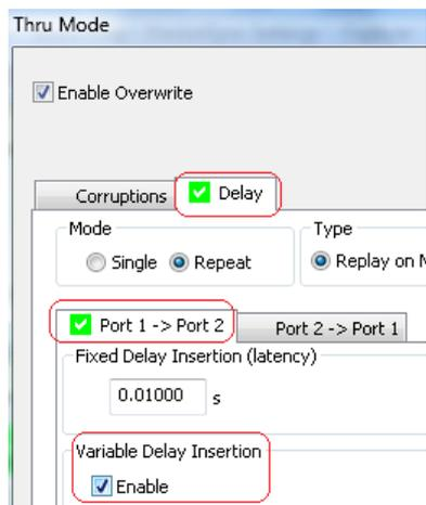
6. Different types of delays can be selected by clicking the appropriate radial button .
