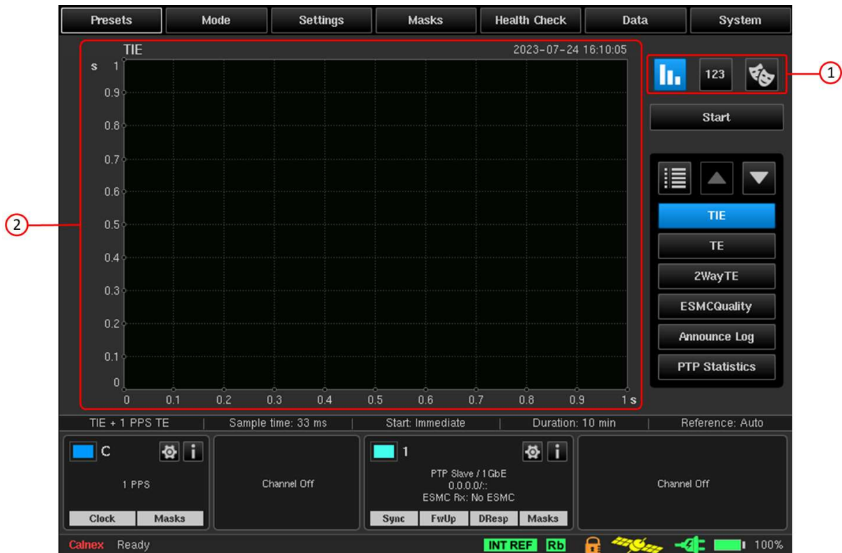
Figure 86 - Main Operating Screen - Viewing Mode Selector Buttons Area and Measurement Graph Window
