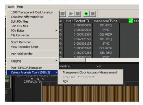
The Calnex Analysis Tool will launch and display the Time Error metrics tab. This will include the metrics Time Error, Avg Time Error (cTE) and Dynamic Time Error.
