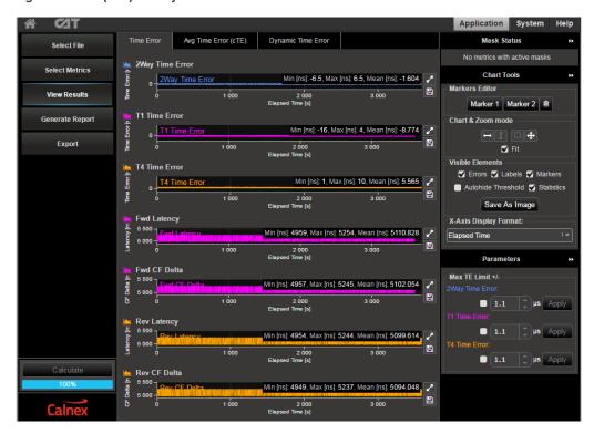
The key measurement for T-TC Time Error is the 2Way Time Error result for the above metrics. Focus should be placed on the analysis of this result.
