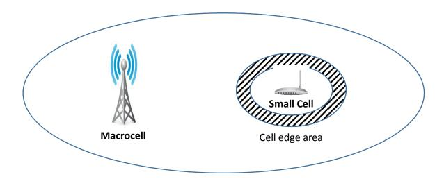
The co-ordination of the almost blank sub-frames requires some level of phase synchronization between the macrocell and the small cell. There is no exact specification for this phase synchronization, since there is no point at which the technique stops working – it just degrades in efficiency to the point where it no longer achieves any performance gain.
