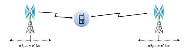
An error in the alignment of these pilot signals is perceived by the handset as a basestation being either nearer to or further away than it actually is. A 3µs time error is the equivalent of a 1km difference in distance.
