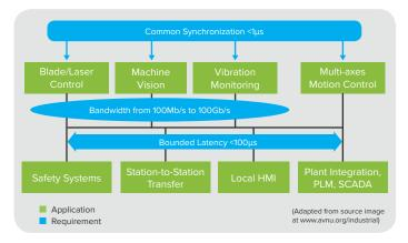
Synchronization is inherently required for many industrial applications, for example to allow real-time data recording and/ or precise sequencing of events. Equipment participating in these applications should be time aligned to better than 1 $\mu$ s across the network.
