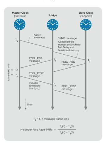
Peer Delay messages yield four timestamps (t1, t2, t3 and t4), from which it is possible to calculate the round-trip time for messages from the initiator to responder, and back, and ultimately the path delay.
