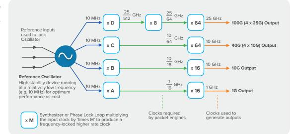
Conceptual example of the clock generation inside a switch or router
